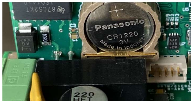
Pic. 4: The placement of the battery holder for RTC.
