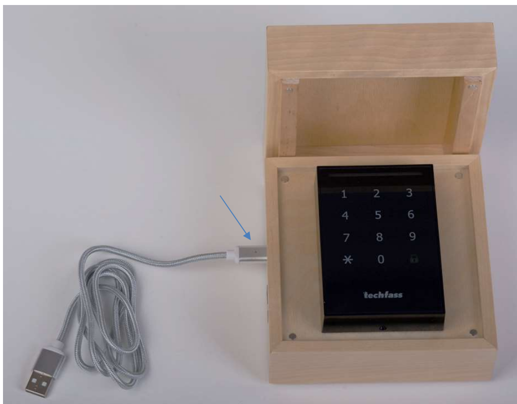
Picture 2: USB cable must be connected with LED up to the Cube. If it is connected upside down, there will be still the power for the reader, but no data will be able to be exchanged between the reader and PC.
