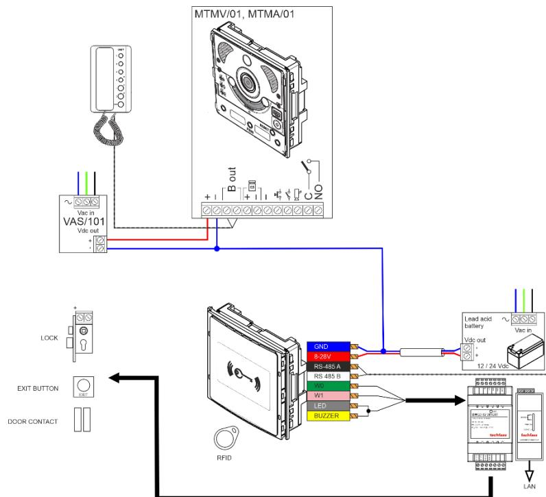
When connecting the WREM 81 MTM( VR) to the MTM entry panel, you can use your own access control system power supply. Connect the wiegand interface & power supply (minimum), and if possible, the signal for LED and buzzer control and bring the RS 485 wires to an accessible place for possible update fw or configuration.
