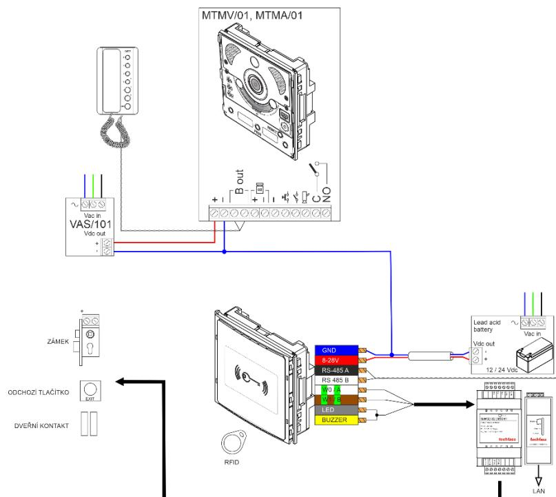
When connecting the WREM 82 MTM(VR) to the MTM entry panel, you can use your own access control system power supply. Connect the wiegand interface & power supply (minimum), and if possible, the signal for LED and buzzer control and bring the RS 485 wires to an accessible place for possible update fw or configuration.
