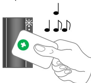
Read the programming card for inserting 5 times in a row; the reader will go into *Deleting cards "above or below"* mode indicated by fast flashing of yellow LED.
