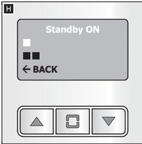
The ▲▼ buttons allow you to scroll and simultaneously view the available brightness levels for Standby mode.
