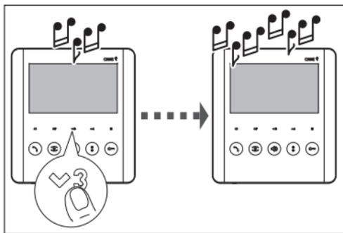
Press the button to select the desired internal receiver.
