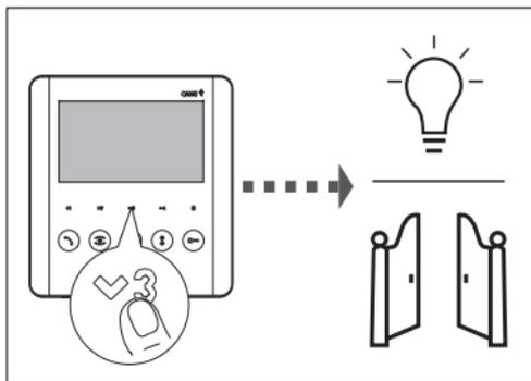
Press the AUX button to activate the desired auxiliary command, for example switching on a light or opening the gate.
