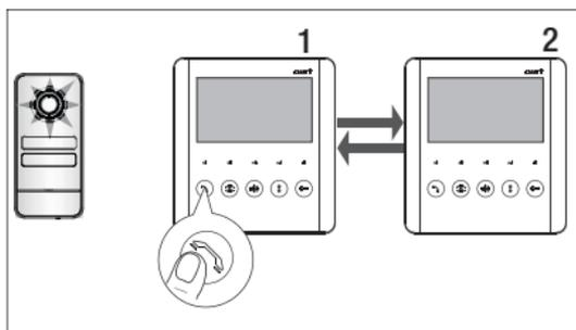
To allow internal receiver 2 to communicate with the entry panel, press this button on internal receiver 1.
