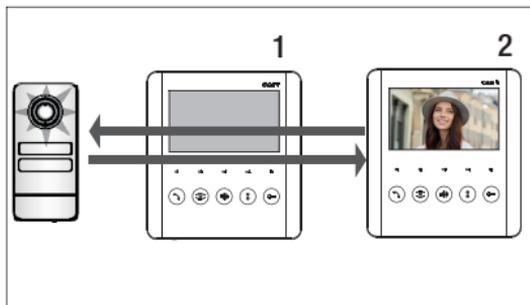
Internal receiver 2 will be able to communicate with the entry panel. The internal receiver with the incoming call can transfer it.
