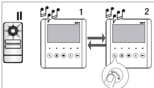
To activate audio communication between two internal receivers, press this button on the called receiver. The entry panel will be put on hold.
